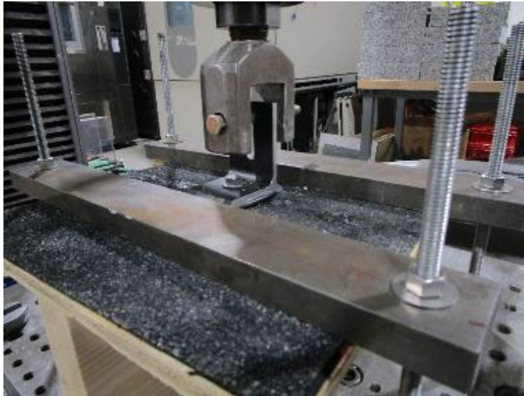
Photo No. 1 Uplift Testing
