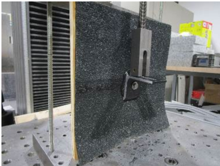
Photo No. 2 Shear Parallel to the Rafter
